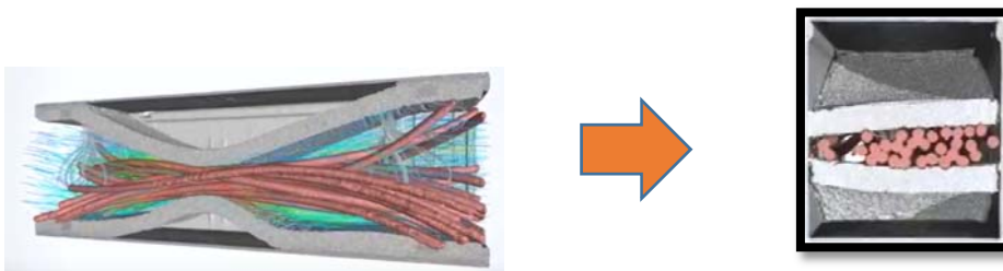
Fig. 8: Competitive pathway device with rubber band around intumescent liner pads to adjust to cable penetrants – third-party CFD simulation by Paul Scherrer Institute from June 2016
