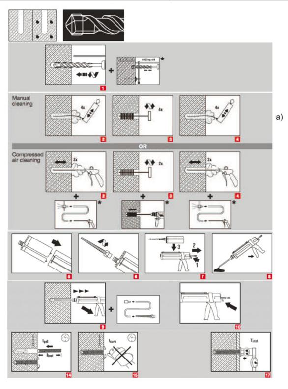
**a) Note:** Manual cleaning for HIS-(R)N M8 and HIS-(R)N M10 only! **b) Note:** Extension and piston plug needed for overhead installation!
